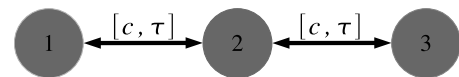
FIG. 8. Schematic representation of the relay mechanism. Oscillators 1 and 3 are coupled bidirectionally to oscillator 2 with time delay \tau and coupling c . There is no direct coupling between 1 and 3.
